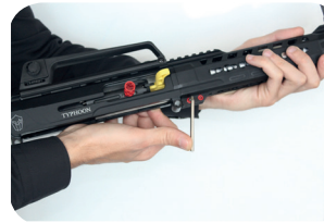
Photo 11-) Use the 4.00 mm allen wrench in your F12 tool set for turning the screws on bottom side of forend for starting to disassemble forend of your shotgun.
