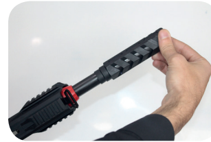
Photo 4-] Turn F12 muzzle break by using your hand to direction of clockwise until thread on barrel allows to disassemble muzzle completely.
