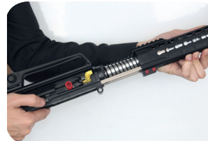
Photo 12-) You can pull easily forend of F12 as in the photo ,if you operated the process in Photo 11.
