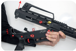
Photo 8-) You will be able to separate upper and lower frame of your gun after these steps as in the photo easily in right way.
