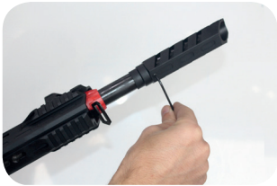
Photo 3-] Turn allen wrench to the direction of clockwise for starting to disassemble F12 muzzle break as in the photo
